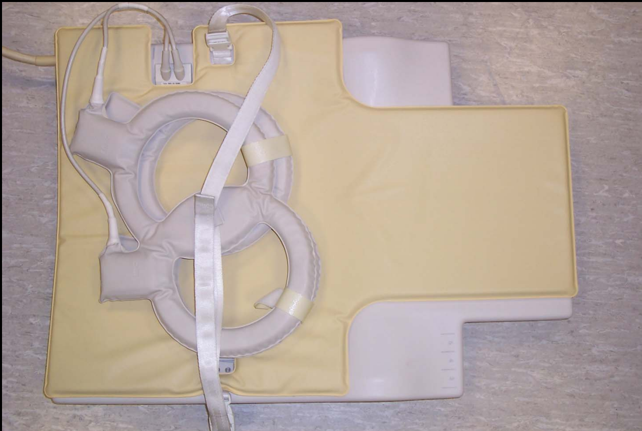
Sense Cardiac Coil with five elements
